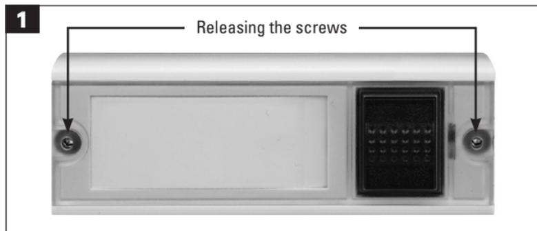
Release the screws of the cover of the wireless doorbell button with the Allen key to remove the top.
