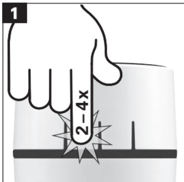
In the default state, press the **select button 2, 3 or 4 times** at an interval of one second to activate the snooze function for **1, 3 or 9 hours**.
