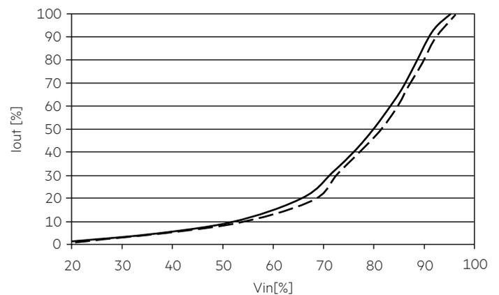
Remark: Dimming curve based on DIMMER ELKO 315GLE!
