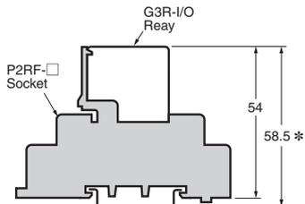
\* These are values when using the DIN track PFP-□N. Heights become higher by approximately 9 mm when using PFP-□N2.
