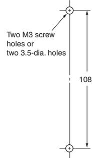
**Note:** Pull out the hooks to mount the Socket with screws.
