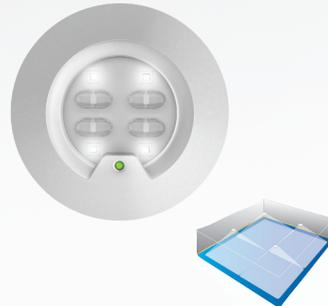
**eFocus, Open Area light distribution**, enables installations for large areas where no fixed escape route is defined, meaning that the complete area must be illuminated. A maximum spacing of up to 24.9m between luminaires reduces the number of required light points and an application range from 2.5m up to 30m for 0.5Lux, enables mounting at the normally occurring heights.
