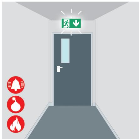
An evacuation order (fire, danger or climatic risk) triggers the **Increased Affordance** function which enables better recognition of the escape route through blinking or pulsing.
