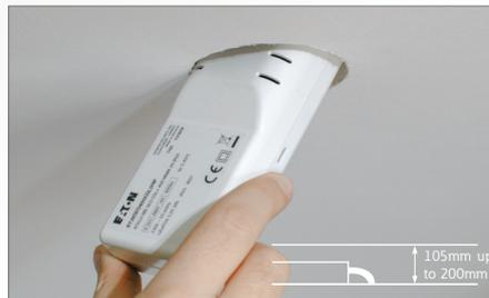
... via standard hole saw (Ø 64-78mm) and lean PSU.
