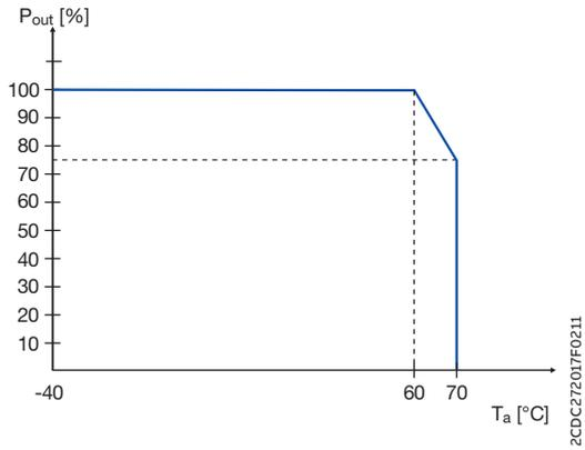
Characteristic curve of temperature at rated load
