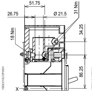
Front for copper/aluminum cables - FC CuAl 2x120 mm<sup>2</sup>
