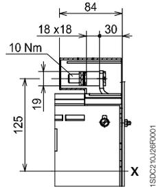
Front for copper/aluminium cables - FC CuAl
