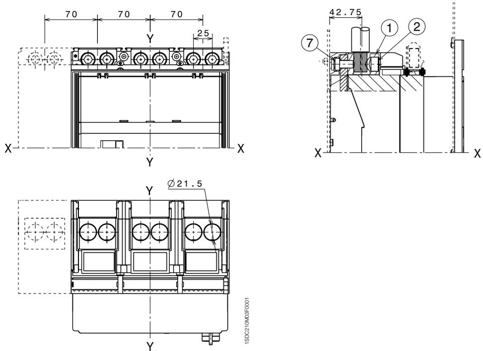
Front for copper/aluminium cables - FC CuAl 4x240 mm<sup>2</sup>
