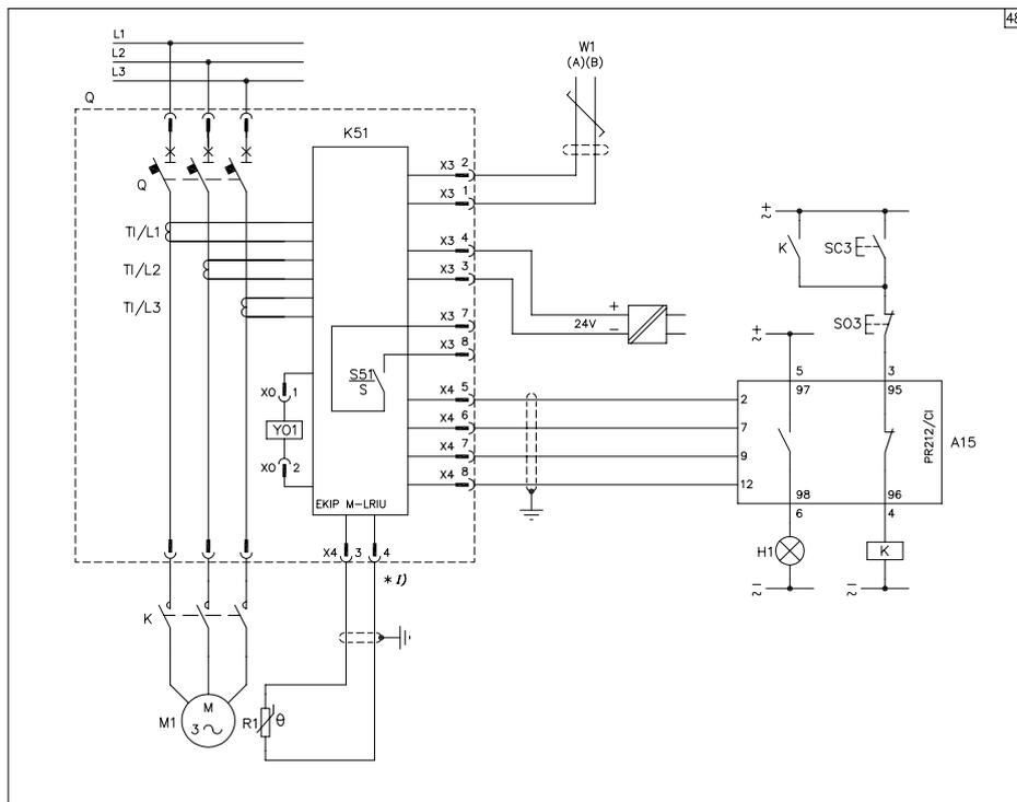
Ekip M-LRIU electronic trip unit connected to PR212/CI contactor control unit and to AF series contactor
