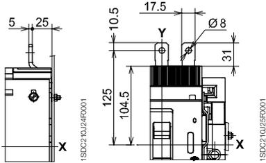
Front for copper cables - FC Cu
