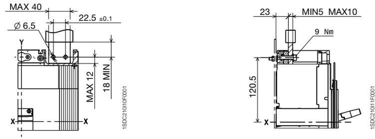
Front for copper/aluminium cables - FC CuAl 2x240 mm<sup>2</sup>
