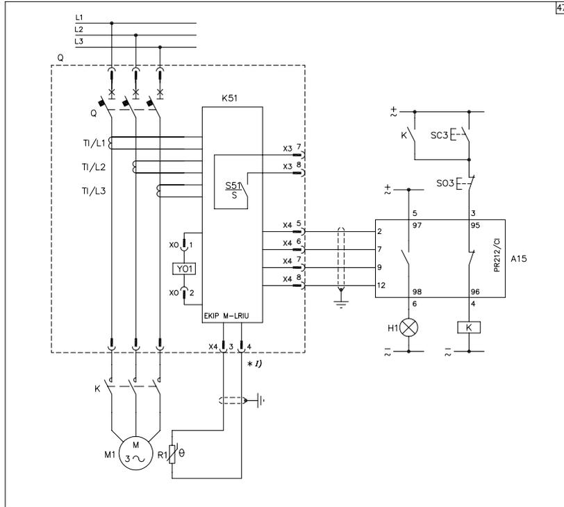
Ekip M-LRIU electronic trip unit with auxiliary supply connected to PR212/CI contactor control unit with MODBUS RS485 communication option
