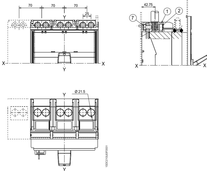
Front for copper/aluminium cables - FC CuAl 4x240 mm<sup>2</sup>
