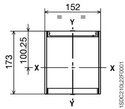
**Drilling template for the compartment door**
