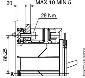
Front for copper cables - FC Cu
