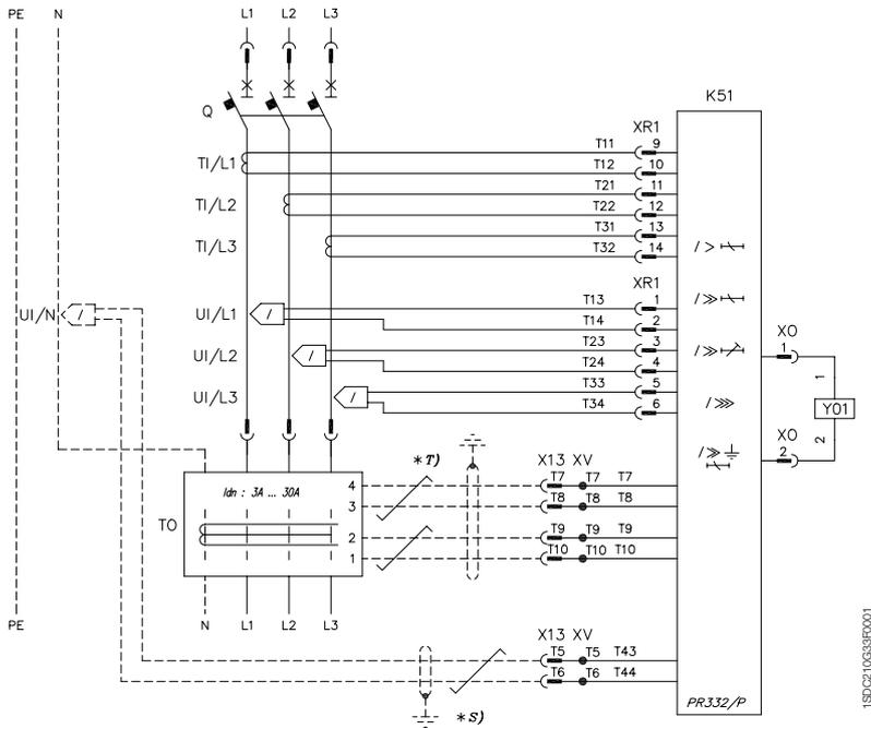
Three-pole circuit-breaker with PR332/P electronic trip unit, residual current protection and  $U \leq 690$  V
