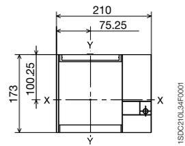
**Drilling template for compartment door and fitting flange**
