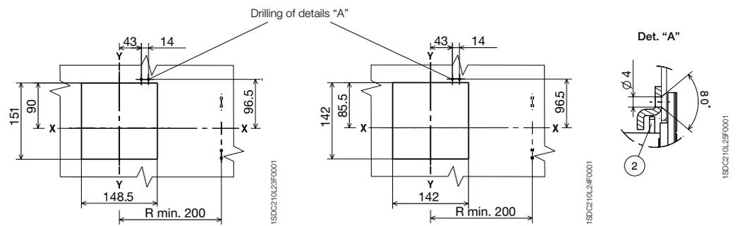
**Drilling template for support sheet**
