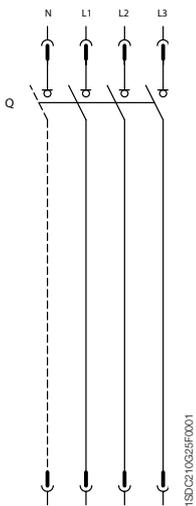
Three- or four-pole switch-disconnector
