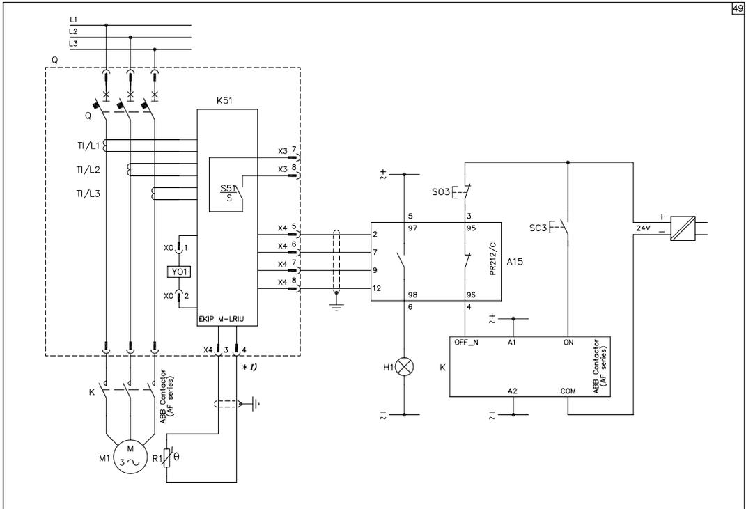
Ekip M-LRIU electronic trip unit with auxiliary supply connected to PR212/CI contactor control unit and AF series contactor with MODBUS RS485 communication option
