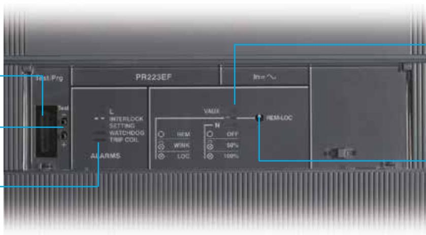
LED signalling the status of the circuit-breaker
