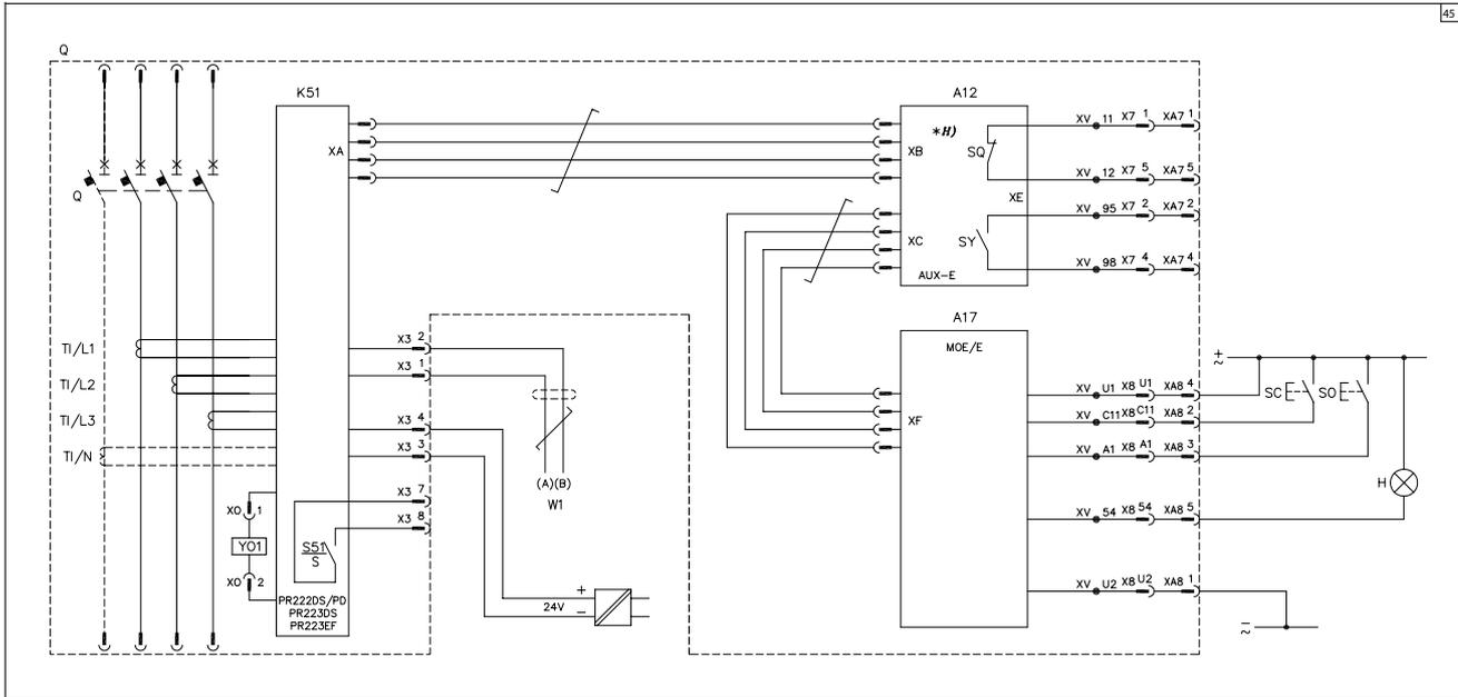
PR22DS/PD, PR223DS or PR223EF electronic trip unit connected with the FDU front display unit and with the AUX-E auxiliary contacts
