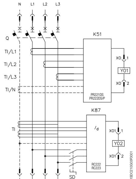
Three-pole or four-pole circuit-breaker with PR221DS, PR222DS/P or PR222DS/PD electronic trip unit and RC222 or RC223 residual current trip unit (for T4, T5 and T6 four-pole only)
