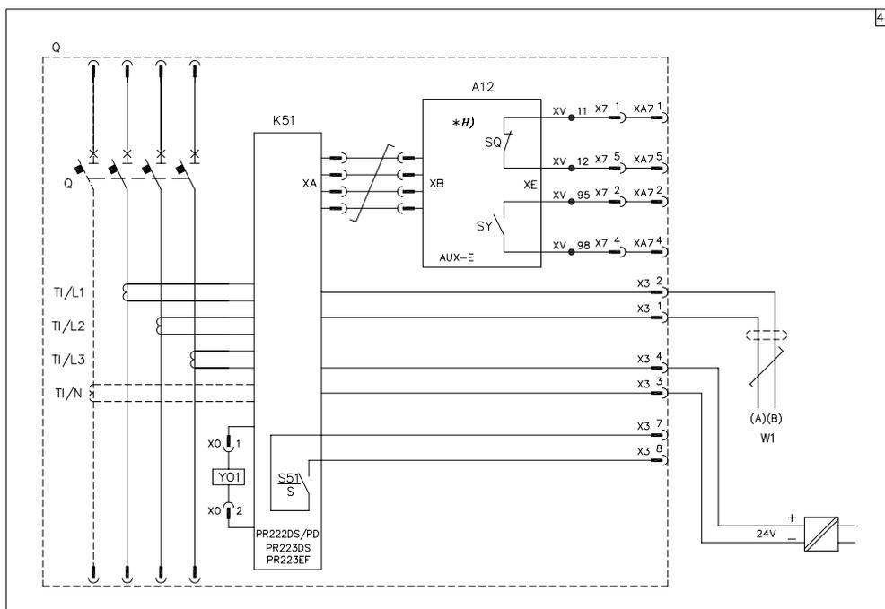
PR22DS/PD, PR223DS or PR223EF electronic trip unit connected with the AUX-E auxiliary contacts and the MOE-E actuation unit
