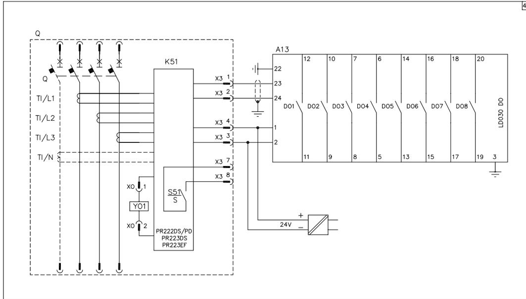
PR222DS/PD, PR223DS or PR223EF electronic trip unit connected with the AUX-E auxiliary contacts
