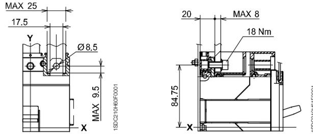
Front for copper cables - FC Cu
