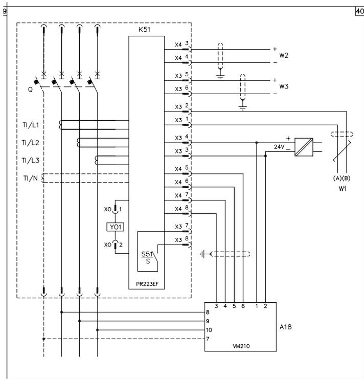
PR222DS/P, PR222DS/PD, PR223DS or PR223EF electronic trip unit connected with the FDU front display unit
