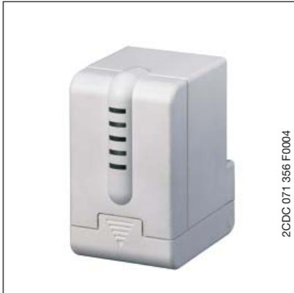
The Electromotor Valve Drive ST/K 1.1 is a proportional valve drive for controlling heating valves via the ABB i-bus® KNX. The valve drive is mounted on thermostat valve bases. The control is carried out via a continuous KNX room thermostat.
