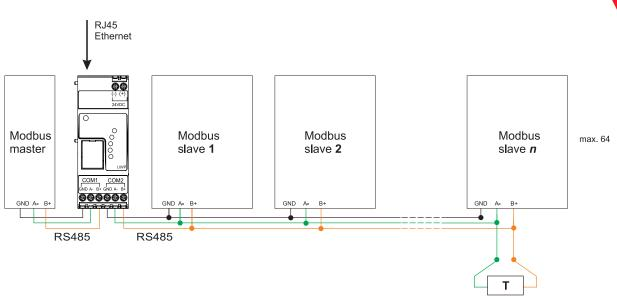
Fig. 2 Modbus RTU connection. COM 1 slave, COM 2 master
