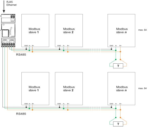
Fig. 1 Modbus RTU connection. COM 1 master, COM 2 master
