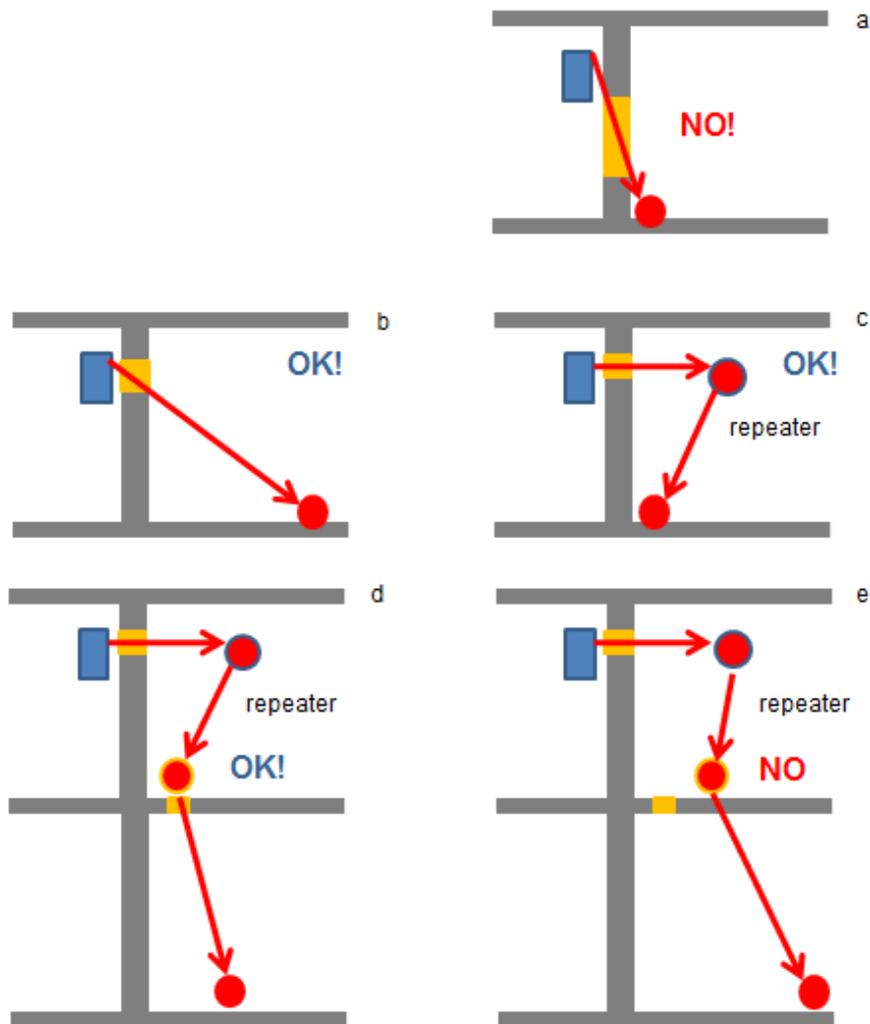
It is also recommended to place a receiver with an internal antenna on the opposite or connecting wall from where the transmitter is placed: this is because near a wall the radio waves might be subject to dispersions and reflections and also because the two antennas should see each other in order to have line-of-sight and the best radio link possible.
