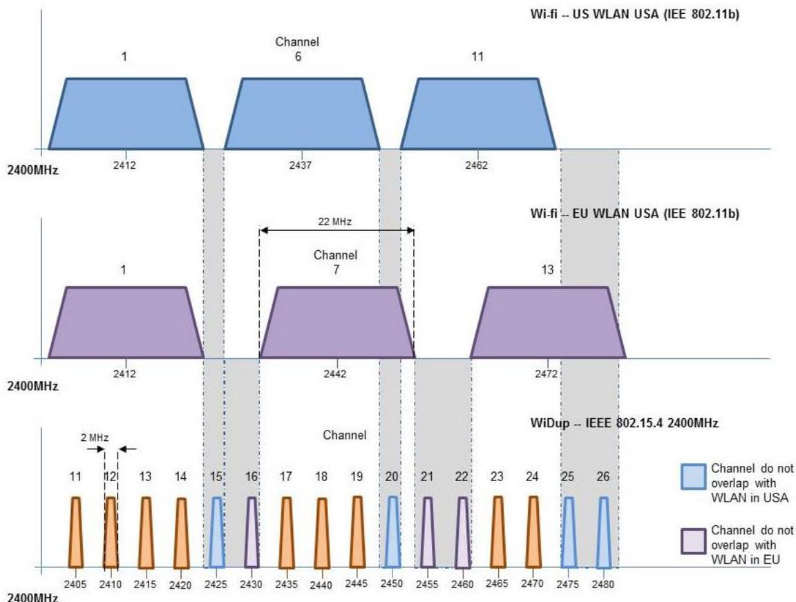
Since channel 15 of WiDup is not overlapping the Wi-Fi bands either in the USA or Europe, it is used by the smart-building system to look for the wireless slave modules present in the field. As for the working band, according to the Wi-Fi channel set in the router, a non-overlapping WiDup channel should be selected: for example, if the router is working on channel 1, channels from 15 to 26 can be selected for the operation of the SH2WBU230N.
