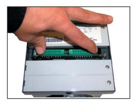
Carefully press to assure that the expansion card is properly connected in the **CVMk2**.
