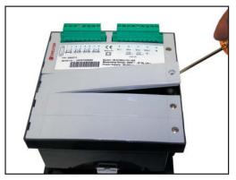
Shut off the power supply to the system. Unscrew and remove the protective cover.
