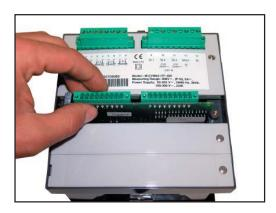
Insert the card by sliding it between the two lateral guides.
