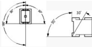
Mechanical shock resistance (IEC/EN 60068-2-27)
