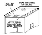
Alarms should be placed in accordance with the general guidelines shown in the diagram above. These recommendations are based on the problem of areas of "dead air" close to corners of rooms and apexes of ceilings, which could result in the prevention of smoke reaching the smoke detector
