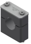
Additional information: The Clamp is made of black, halogen-free and self-extinguishing (grade V0, UL 94) polyprophylene and stainless steel. Fire exposure does not lead to emission of toxic gases. Oxygen index (ASTM D 2863): 307%. The material shows good resistance to chemicals. Working temperature range is -20 to +110° C.
