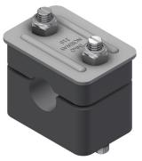
Additional information: The Clamp is made of black, halogen-free and self-extinguishing (grade V0, UL 94) polyprophylene and stainless steel. Fire exposure does not lead to emission of toxic gases. Oxygen index (ASTM D 2863): 307%. The material shows good resistance to chemicals. Working temperature range is -20 to +110° C.
