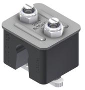
Additional information: The Clamp is made of black, halogen-free and self-extinguishing (grade V0, UL 94) polyprophylene and stainless steel. Fire exposure does not lead to emission of toxic gases. Oxygen index (ASTM D 2863): 307%. The material shows good resistance to chemicals. Working temperature range is -20 to +110° C.
