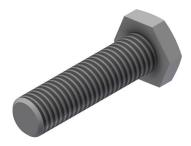
Additional information: Recommended length of the Bolt for U-21 channels is 25 mm when mounting parts with material thickness 5 mm. Recommended length of the Bolt for U-41 channels is 30 mm when mounting parts with material thickness of 5 mm. Increase the length of the Bolt accordingly when mounting parts with more than 5 mm material thickness. Longer lengths in DIN 931 partly threaded. STD: 50
