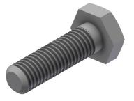
Additional information: Recommended length of the Bolt for U-21 channels is 25 mm when mounting parts with material thickness 5 mm. Recommended length of the Bolt for U-41 channels is 30 mm when mounting parts with material thickness of 5 mm. Increase the length of the Bolt accordingly when mounting parts with more than 5 mm material thickness. Longer lengths in DIN 931 partly threaded. STD: 100
