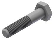
Additional information: Recommended length of the Bolt for U-21 channels is 25 mm when mounting parts with material thickness 5 mm. Recommended length of the Bolt for U-41 channels is 30 mm when mounting parts with material thickness of 5 mm. Increase the length of the Bolt accordingly when mounting parts with more than 5 mm material thickness. Longer lengths in DIN 931 partly threaded. STD: 50
