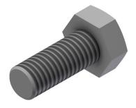
Additional information: Recommended length of the Bolt for U-21 channels is 25 mm when mounting parts with material thickness 5 mm. Recommended length of the Bolt for U-41 channels is 30 mm when mounting parts with material thickness of 5 mm. Increase the length of the Bolt accordingly when mounting parts with more than 5 mm material thickness. Longer lengths in DIN 931 partly threaded. STD: 200
