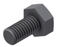
Additional information: Recommended length of the Bolt for U-21 channels is 25 mm when mounting parts with material thickness 5 mm. Recommended length of the Bolt for U-41 channels is 30 mm when mounting parts with material thickness of 5 mm. Increase the length of the Bolt accordingly when mounting parts with more than 5 mm material thickness. Longer lengths in DIN 931 partly threaded. STD: 200
