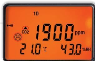
With its large two-colour backlit screen, the **C.A 1510** can be used to measure and display 3 parameters simultaneously (CO<sub>2</sub>, temperature and RH). To make it simpler to use, integrated help is provided for interpretation of the level of comfort based on the CO<sub>2</sub> level and hygrothermal comfort criteria.
