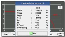
Summary of the electrical data measured (OPC) and the data provided by the manufacturer (STC). The voltage, current and maximum power (MPP) of the installation are also indicated, as are the efficiency (FF), the no-load voltage and the short-circuit current.
