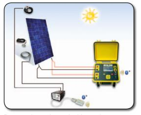
Because the 4-wire method is used to measure the output current and voltage of the solar panels, the results are highly accurate even over considerable cable lengths.
