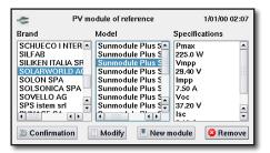
Selection of more than 10,000 manufacturer references stored in the database inside the instrument. It is a simple task to update this list, either directly on the instrument by means of its touch screen, or in your office with the management software delivered with the FTV200.
