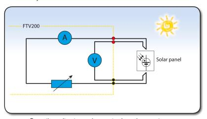
Once the voltmeter and ammeter have been set up on the installation, users can vary the resistance RL, which is the instrument's internal resistance. The voltage and current values from the cells at various points on the solar panels are known, so they can be compared immediately.
