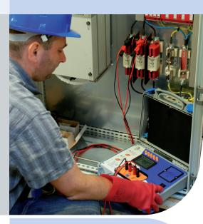
The Euro - Z 290 A is a professional portable test instrument intended for low impedance measurements in environments up to CAT IV /310 V. It can operate alone or in combination with the METREL instruments. High precision line impedance and high precision fault loop impedance measurements in range from 1 m $\Omega$  up to 19.99  $\Omega$  are its excellence.
