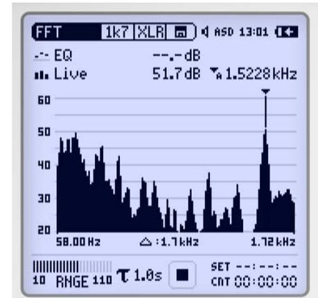
The real-time FFT is the ideal tool for visualization of comb filters and narrow band effects. It measures the actual level and the averaged level Leq in three ranges over the entire audio band.
