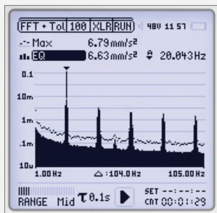
The Vibration Option turns the XL2 into a flexible vibration meter, with FFT analysis and data logging, for frequencies down to 0.7 Hz.
