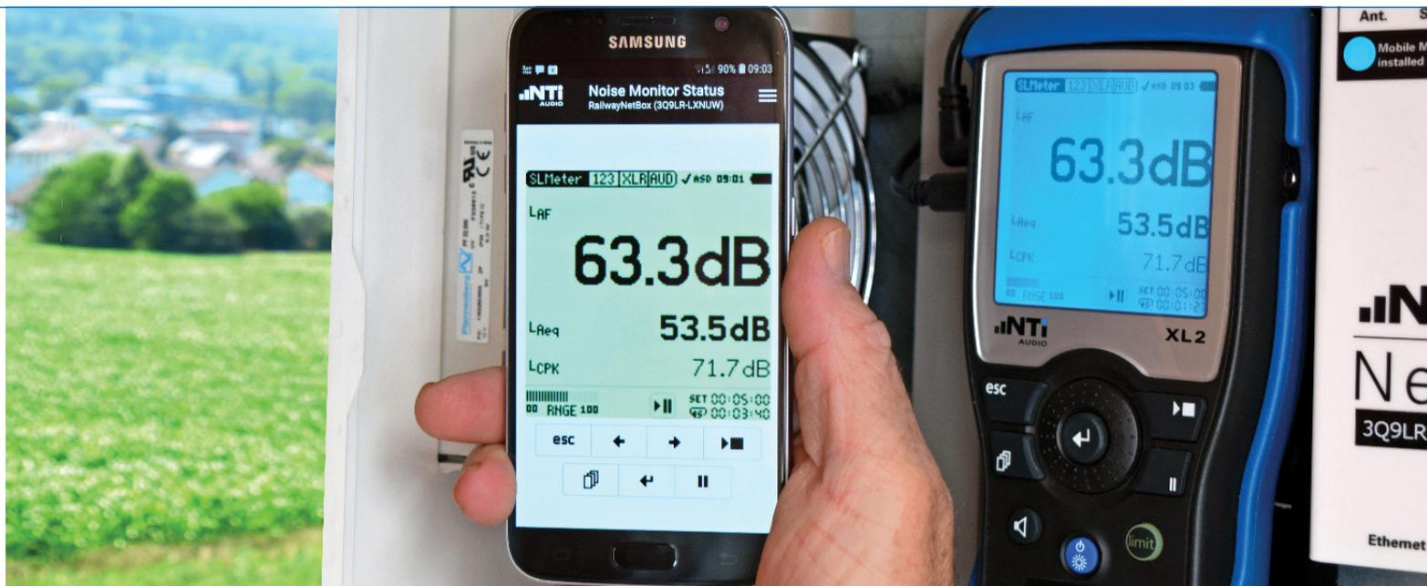
The XL2 Sound Level Meter provides all the functions needed to measure and monitor noise. Its removable SD card offers plenty of space to record levels, spectra and audio files. The data can also be read out during an ongoing measurement via its USB interface.
