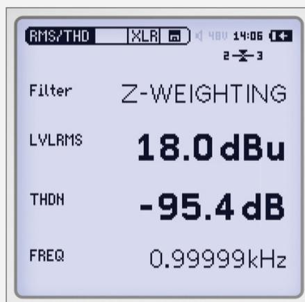
With a balanced XLR and unbalanced RCA input, the XL2 is a high-performance audio analyzer. It simultaneously measures balance, RMS level, frequency, and harmonic distortion (THD + N).
