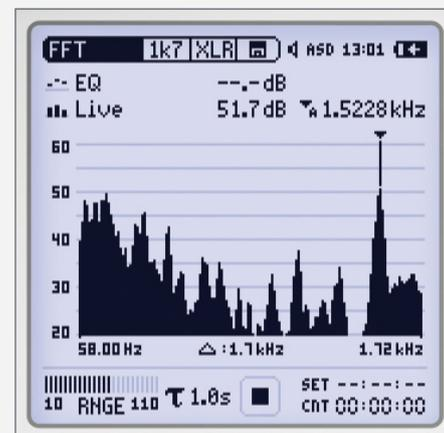
The real-time FFT is the ideal tool for detecting comb filters and resonant frequencies. The XL2 measures the actual level and the time-averaged Leq level in three frequency ranges.
