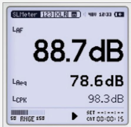
The XL2 with measurement microphone is a precise Sound Level Meter. All measurement results are available simultaneously, e.g. Leq, Lmin, Lmax, and LCpeak, with the frequency weighting A, C, Z and the time weighting Fast, Slow and optional Impulse.
