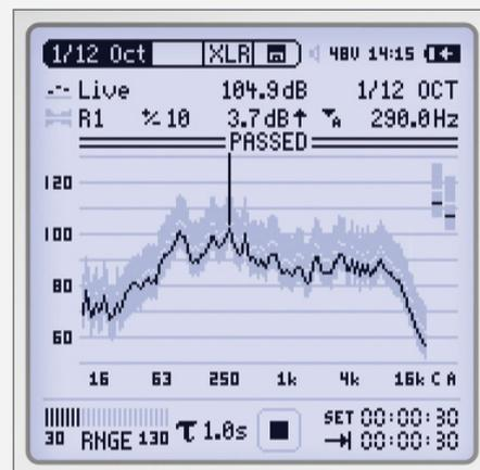
The Spectral Limits Option extends spectral analysis with 1/6 and 1/12 octave resolution, zoom FFT, reference curve recording, relative display, extensive tolerance management for pass/fail testing, and Noise Curves.
