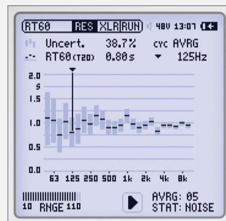
Measure the reverberation time in a room with automatic triggering from an impulse or gated pink noise sound source.
