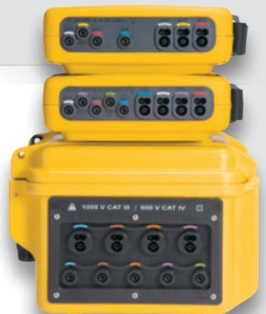
Designed to cover all 600 V CAT IV and 1000 V CAT III applications in compliance with the IEC 61010 standard, the Qualistar+ range is divided up according to the functions provided and the connections available:
