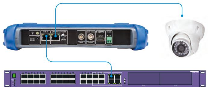
Power the camera by passing PoE+ from the network and through the tester - RJ45 port.
