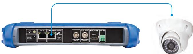
Power the camera using Power over Ethernet (PoE+), up to 24 watts from the tester - RJ45 port.
