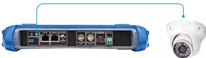
Power the camera using 12V DC from the tester - 2.5mm to 3.5mm barrel connector.
