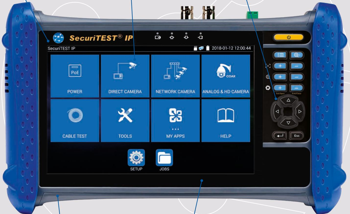
**Long battery life** - Up to 10 hours continuous usage with a lithium-Ion battery.
