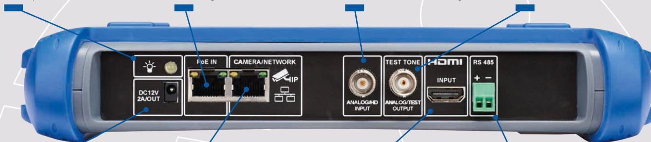
**12V DC power supply** - Power any camera using the built-in 12V/2A DC power supply.
