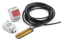
The RAYSTAT-M2-R-SENSOR is designed for mounting in gutters and drain pipes. RAYSTAT-M2-R-SENSOR detects moisture, while RAYSTAT-M2-A-SENSOR detects temperature. The snow melting system will be energised only when the outdoor temperature is below the selected setting and moisture is detected on the RAYSTAT-M2-R-SENSOR.
