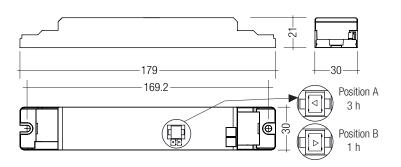
Note: LED Driver supplied with duration link in 3 hours position. Duration link must be set before battery and mains connection. The EM converterLED ST 134 NiCd is supplied without a duration link.
