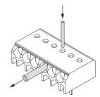
Loosen wire through twisting and pulling or using a Ø 1mm release tool
