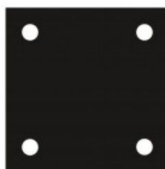
Dampsperre for betongfundament c/c 290 mm
