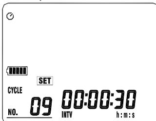
12. Press ◀ key to complete the action and to enter the auto-cycle timer datalogging mode, the “CYCLE” mark is flick displayed.
