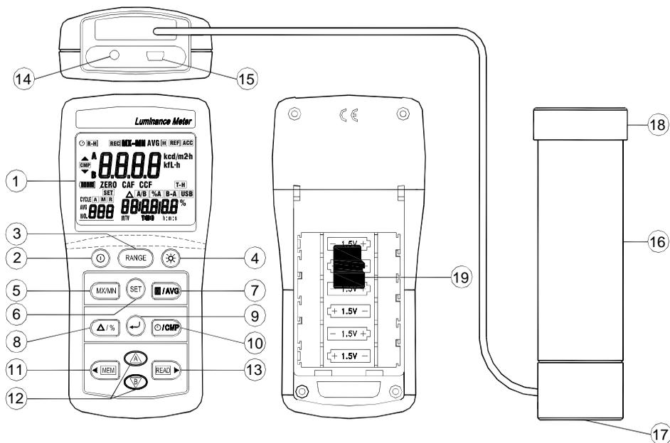
**1. LCD Display:** 4 digit display with a maximum of 9999 readings and the indicating signs of measured values, unit function symbols and decimal points etc. are displayed.
