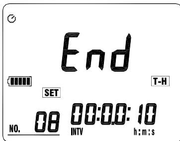
12. Press ← key to complete the action and to enter the no-cycle timer datalogging mode, the “T-H” mark is flick displayed.
