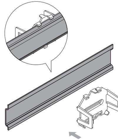
**Step 1:** Clip the mounting clip onto DIN rail.
