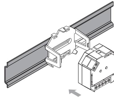
**Step 2:** Install the device onto the mounting clip in the correct direction.
