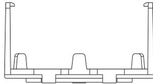
This DIN rail mounting clip is developed to mount the mini in wall module on a 35mm DIN rail. It is applicable to all devices with the casing design as follows:
