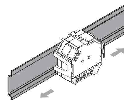
**Step 3:** The device can slide freely on the DIN rail.
