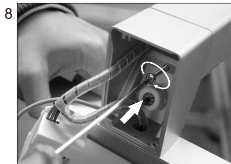
Fix the lamp holder with screws-3
