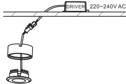
3. Fix the mounting base to the cabinet with screws. Push the luminaire up into mounting base. Ensure that it is securely located.
