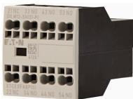
**Auxiliary contact module, 4 pole,  $I_{th}=16\text{ A}$ , 3 N/O, 1 NC, Front fixing, Push in terminals, DILM7 - DILM15**
