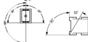
Mechanical shock resistance (IEC/EN 60068-2-27)
