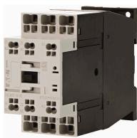
Contactor, 3 pole, 380 V 400 V 7.5 kW, 1 N/O, 1 NC, 230 V 50 Hz, 240 V 60 Hz,
