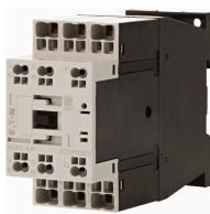
Contactor, 3 pole, 380 V 400 V 11 kW, 1 N/O, 1 NC, RDC 24: 24 - 27 V DC, DC operation, Push in terminals
