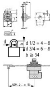
Minimum door coupling rotary handle clearance from door pivot point
