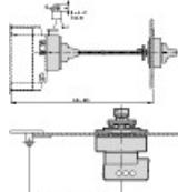
Minimum door coupling rotary handle clearance from door pivot point
