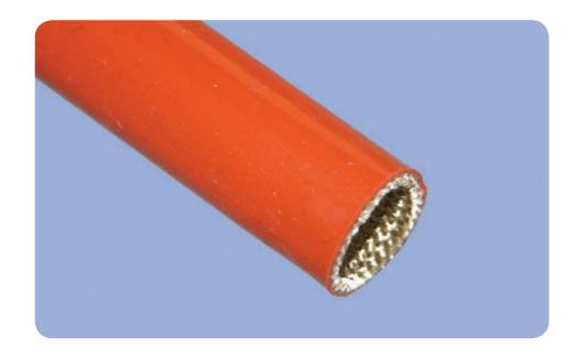
**GES** is a braided fiberglass sleeve with a silicone rubber coating designed to provide electrical insulation. The thickness of the silicone coating determines the dielectric strength, which ranges from 4 to 10 kV.
