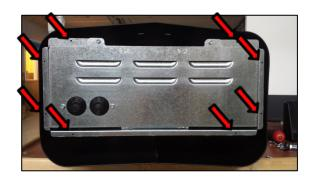
2. Lay the heater down to easier acces the underside. Mount the legs with the small screws in these 8 holes.
