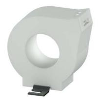
Residual-current transformer for residual current monitoring Bushing opening 35 mm Residual current 30 mA...40 A  $\,$
