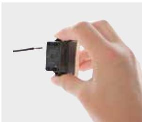
1. Strip the cable about 14 mm and introduce it into the terminal.
