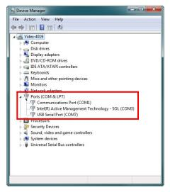
Select 'USB Serial Port (COM7)' from the expanded list and 'double click'. The 'USB Serial Port (COM7) Properties' window will appear. The 'General' Tab will already be selected and display the following information. Ensure that the information displayed is the same as the information highlighted.
