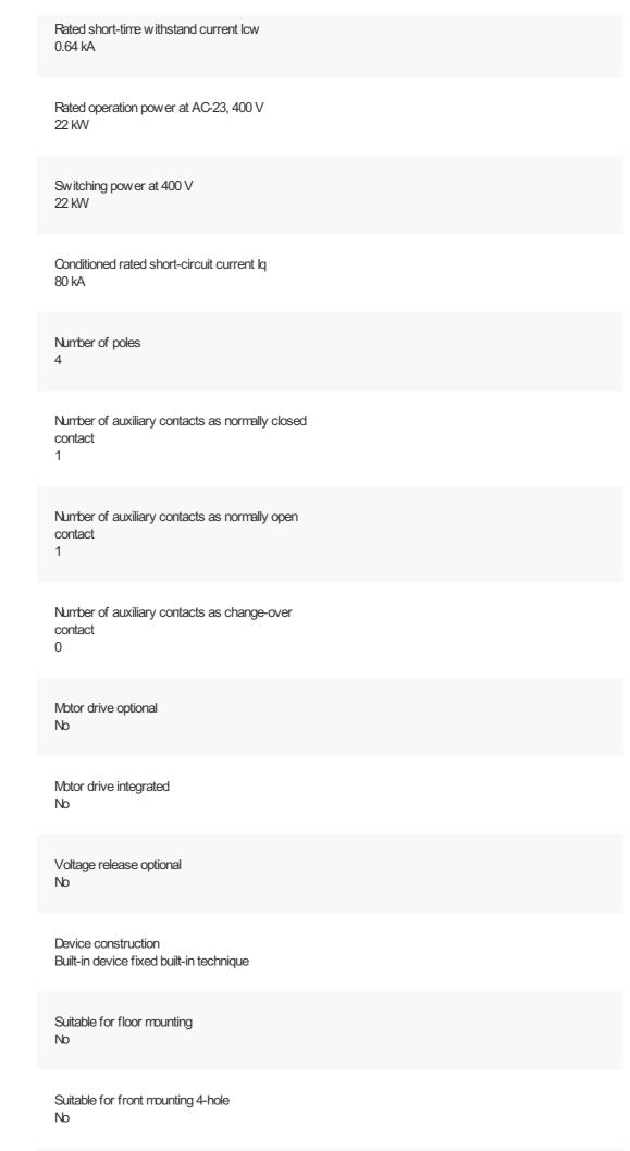
Suitable for front mounting centre Suitable for distribution board installation Suitable for intermediate mounting No Colour control element Black Type of control element Door coupling rotary drive Interlockable Yes Type of electrical connection of main circuit Screw connection Degree of protection (IP), front side IP65 Degree of protection (NEVA)
