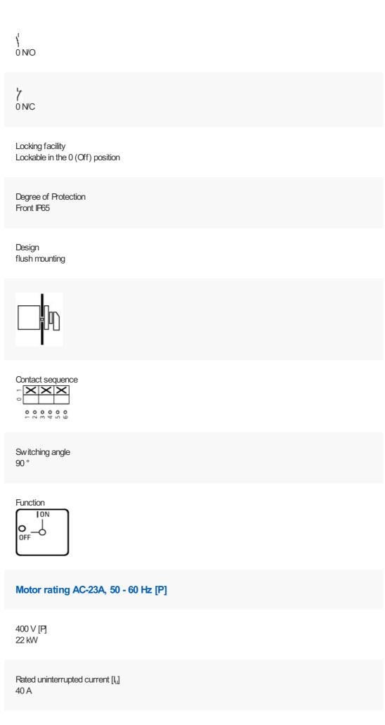
Note on rated uninterrupted current  $I_u$  Rated uninterrupted current  $I_u$  is specified for max. cross-section.
