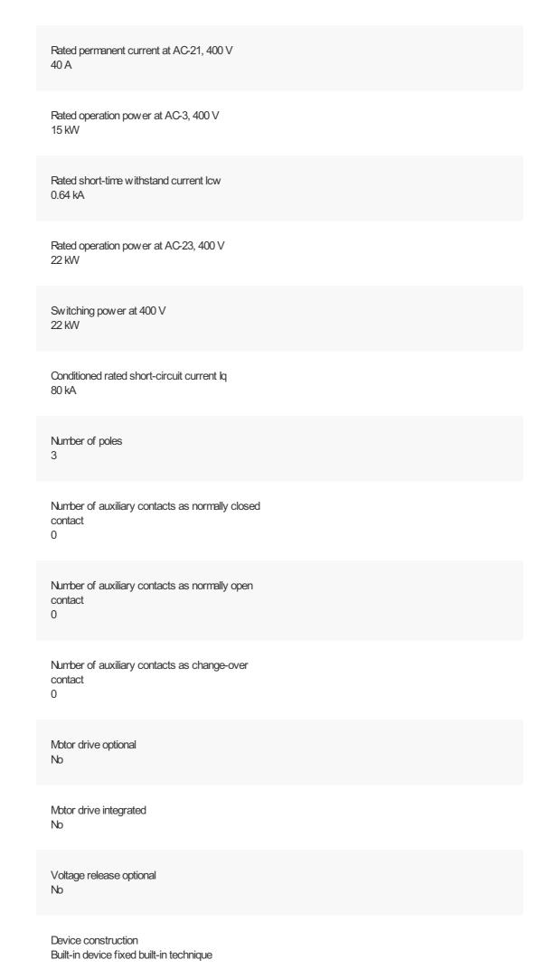
Suitable for floor mounting Suitable for front mounting 4-hole Suitable for front mounting centre Suitable for distribution board installation No Suitable for intermediate mounting Colour control element Black Type of control element Door coupling rotary drive Interlockable Yes Type of electrical connection of main circuit Screw connection Degree of protection (IP), front side IP65 Degree of protection (NEVA)
