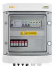
**DC+AC connection combiner box with 1000V surge arrester type 2, 2 x PV string, 2 x MPPT // surge arrester AC type 2, 20A 3-F, RCD type A 100mA 40A**
