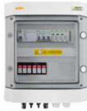
**DC+AC connection combiner box with 1000V surge arrester type 1+2, 2 x PV string, 2 x MPPT // surge arrester AC type 1+2, 32A 3-F, RCD type A 40A 300mA**
