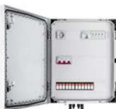
**DC+AC connection combiner box IP66 with 1000V surge arrester type 2, 4 x PV string, 4 x MPPT // surge arrester AC type 2, 100A 3-F, FR 100A, phase sig. + socket (SE 50kW )**
