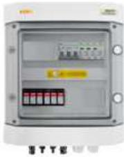
**DC+AC connection combiner box with 1000V surge arrester type 1+2, 2 x PV string, 2 x MPPT / surge arrester AC type 1+2, 40A 3-F**
