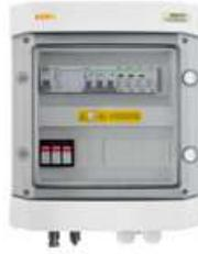
**DC+AC connection combiner box with 1000V surge arrester type 1+2, 1 x PV string, 1 x MPPT // surge arrester AC type 1+2, 16A 3-F, RCD type A 100mA 40A**
