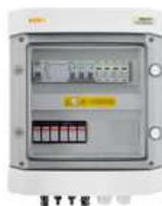
**DC+AC connection combiner box with 1000V surge arrester type 2, 2 x PV string, 2 x MPPT // surge arrester AC type 2, 16A 3-F, RCD type A 100mA 40A**
