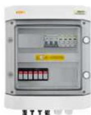
**DC+AC connection combiner box with 1000V surge arrester type 2, 2 x PV string, 2 x MPPT // surge arrester AC type 2, 20A 3-F, RCD type A 300mA 40A**
