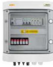
**DC+AC connection combiner box with 1000V surge arrester type 1+2, 2 x PV string, 2 x MPPT // surge arrester AC type 1+2, 16A 3-F, RCD type A 100mA 40A**
