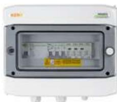
**Connection combiner box with AC surge arrester type 1+2, 20A 3-F, RCD type A 40A 300mA**
