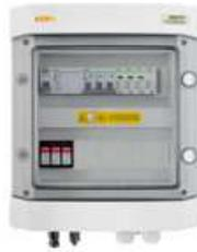
**DC+AC connection combiner box with 1000V surge arrester type 1+2, 1 x PV string, 1 x MPPT // surge arrester AC type 1+2, 10A 3-F, RCD type A 100mA 40A**
