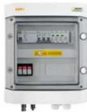
**DC+AC connection combiner box with 1000V surge arrester type 1+2, 1 x PV string, 1 x MPPT // surge arrester AC type 1+2, 10A 3-F, RCD type A 40A 300mA**
