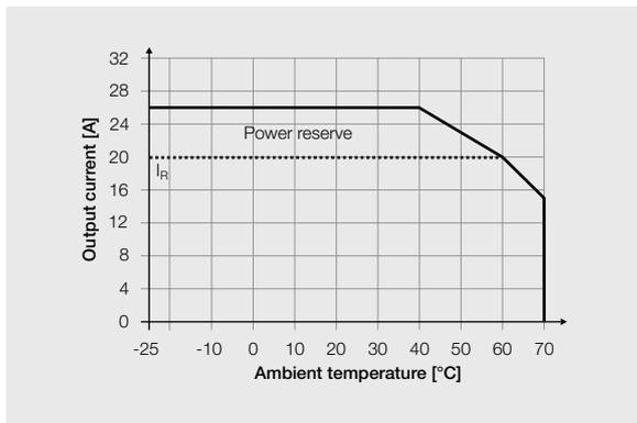
Characteristic curves of temperature at U<sub>out</sub> = 24 V, mounting position 1
