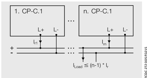
Simple redundancy or n+1 setup
